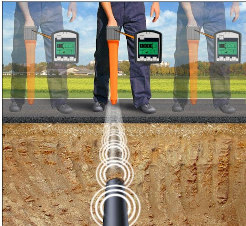
The alignment of the receiver in relation to the orientation of the conductor (the antenna being the starting point of alignment) has the following effects on the reception signal strength:
